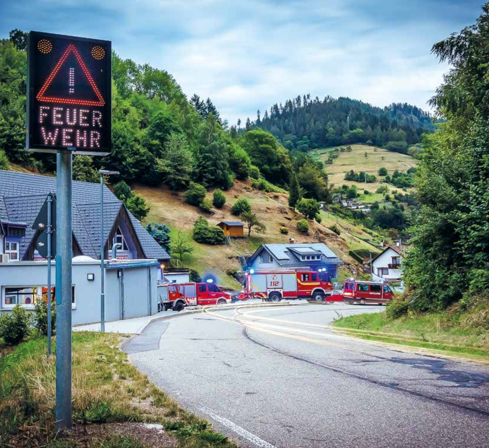
VARIABLE LED TRAFFIC SIGN
