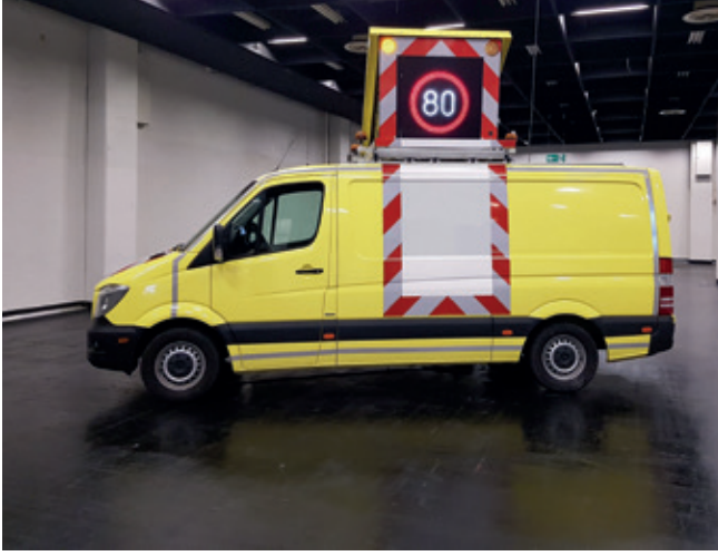
Change signal transmitter rotated 90 degrees on the escort vehicle.
